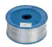
Stranded Aluminium Wire has the lowest resistance allowing long fences to be powered up, reducing the number of energizers needed. The flexibility offered by the stranded aluminium wire construction makes working with this wire easier during installation and results in a neat clean look on the fence without compromising the fence's performance.
